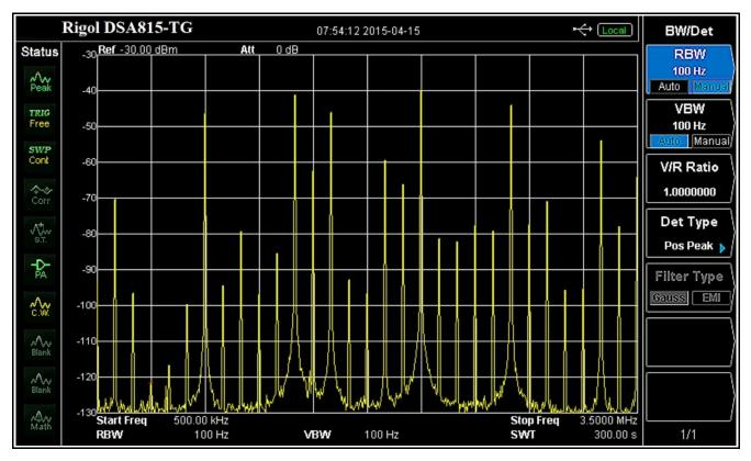
Below is a DSA815-TG display capture of the toroid version of the 1.5 MHz EHP filter being fed 600 kHz and 1100 kHz tones at -6 dBm. The Norton amplifier is NOT in the signal path for the display below.
