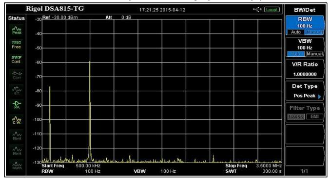
There is not much to see. A very weak spur of about -125 dBm at about 900 kHz is an internal spur of the spectrum analyzer. Whether the other "blips" are spurs, IMD, or just noise floor anomalies I do not know. This shows that the 1.5 MHz EHP filter is IMD free down to about -130 dBm or lower.
