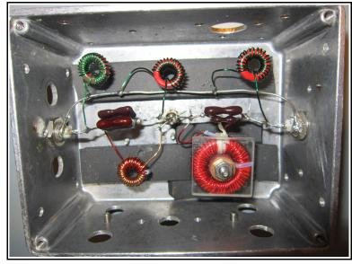
squares of plexiglass which provides secure support and prevents contact with the metal box. There is a 1/2 inch insulated standoff with pronged solder lug on top which is used for soldering together the middle leads of the capacitor pairs. The end leads of the capacitors are soldered directly to the BNC center conductors. The correct
